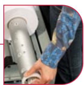
Easy loading of 2" and 3" cores
